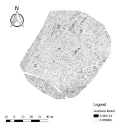
**Figure 4.** "Goodness for fit" map considering a *thresholding* of 0.65 and a *minsize* of 100, with separated bands.
