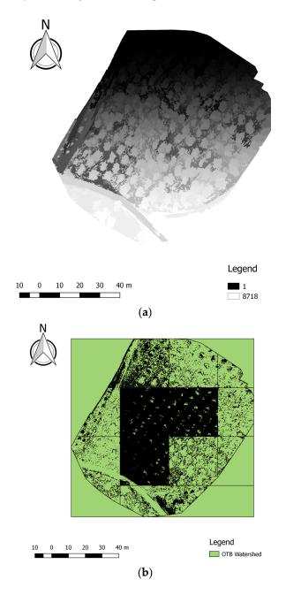
Figure 3. (a) Segmentation with *i.segment* algorithm; (b) segmentation with *Watershed algorithm*.
